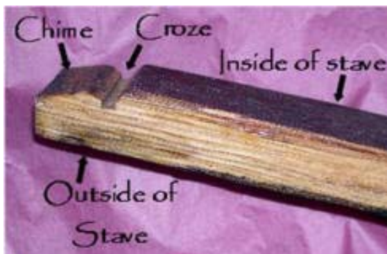
A "croze" or groove is cut in the staves to fit into the barrel heads.
